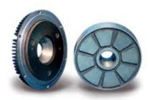
The permanent magnet magnetizes the induced plate, thus generating a ring of alternating polarity and the magnetic forces required to transmit the torque.
