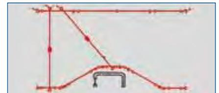
Articulated connections ensure that the crane girder cannot snag. Single-girder cranes can also travel on angled or converging crane runways.
