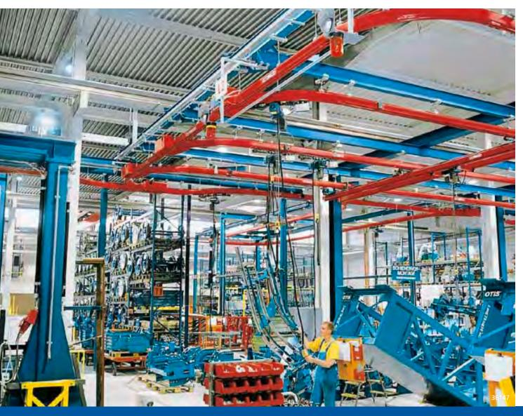
Cable trolleys can also be used to suspend hoses for transporting fluids or gases.
