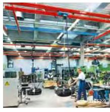
KBK double-girder suspension cranes also feature a low deadweight and favourable structural dimensions. In addition, the pendulating suspension largely absorbs the horizontal forces caused by starting, braking and stopping. They can even be installed in buildings of light steel construction.
