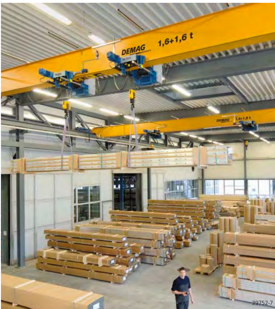
Two EKDR monorail hoists transporting aluminium profile sections in tandem operation.
